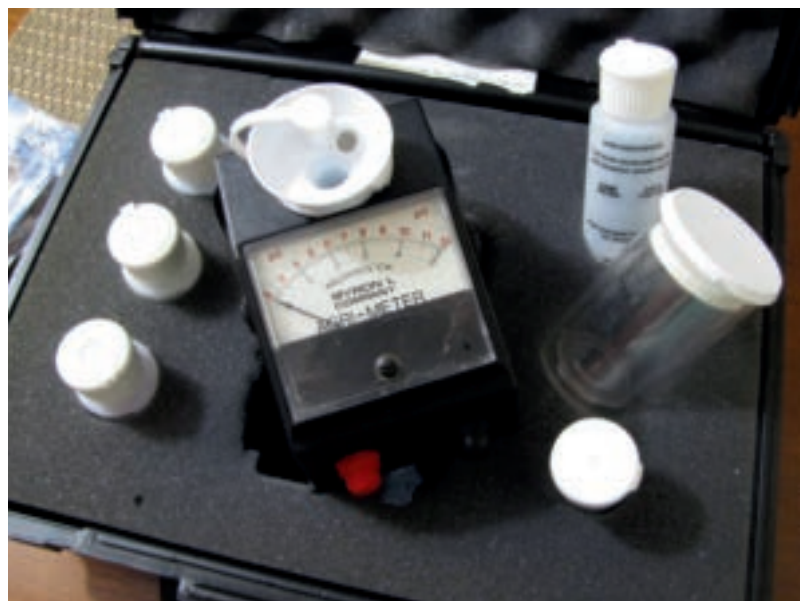
Figure 20. Soil testing equipment used for pH and EC monitoring.
