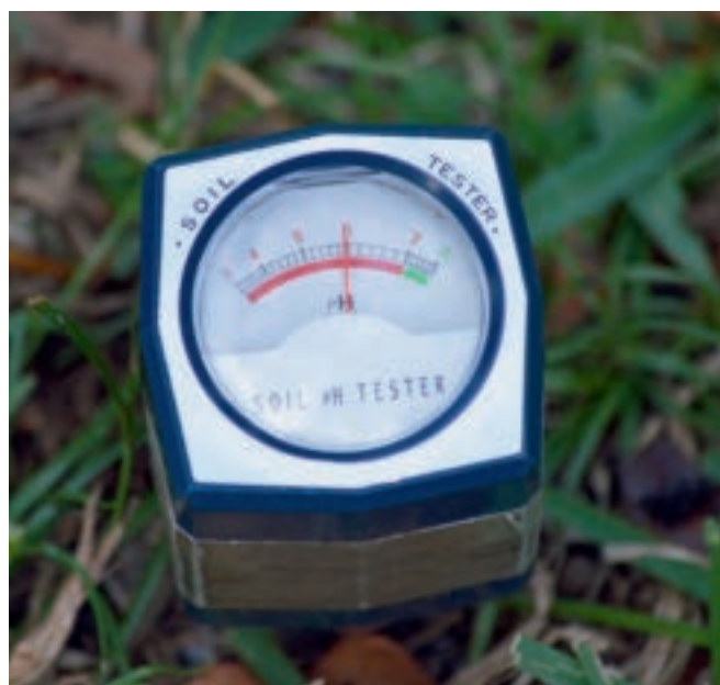
Figure 14. Inexpensive soil test meter for the field.
